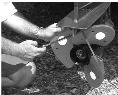
**2.** Secure blade covers with the rubber cinch strap stretched onto all three locking tabs. This holds the blade covers securely together for trailering.
