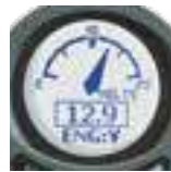
as a volt meter for single engine
